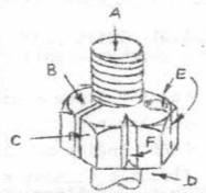
A. Hacksaw down bolt and through nut in direction A
