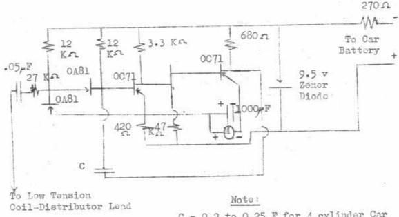
C = 0.2 to 0.25 F for 4 cylinder Car C = 0.3 to 0.35 F 6 cylinder Car M = 0.5 Milliammeter.
