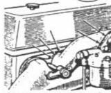
Air leaks in induction manifold, butterfly spindle bearing or cylinder head gasket
