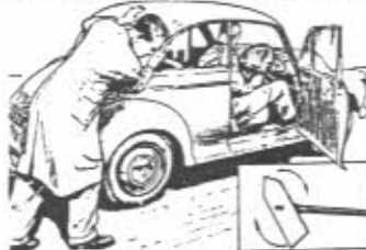
With a helper to push the car forward you can easily check the cable turns per mile to see if you've got the right speedo head.
