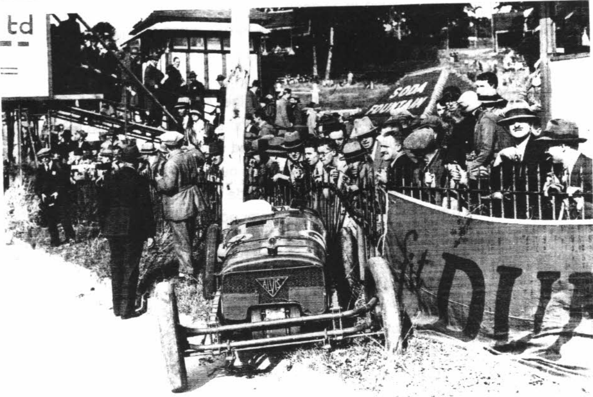
Hors de combat: C. M. Harvey, winner of the 1923 200 Miles race, was less fortunate in the 1926 event. His straight-eight front-drive 1½-litre Grand Prix Alvis was baulked on its 23rd lap by a slow 7 hp Fiat at one of the artificial turns. The Alvis spun wide and struck a telegraph pole and iron railings near the timekeepers' box in the finishing straight.
