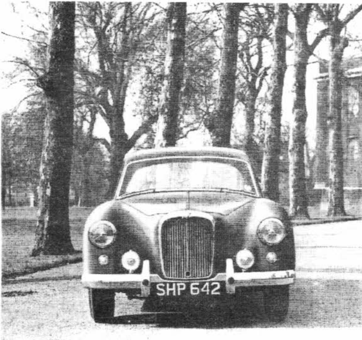
Bumper over-riders have rubber buttons for protection, there are twin fog lamps, and the side lights are mounted separately. Provision is made for a starting handle
