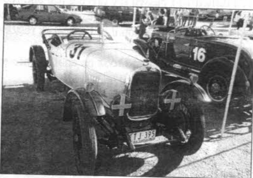
This is the car as it looks today with cycle wings and "frameless" screen.
