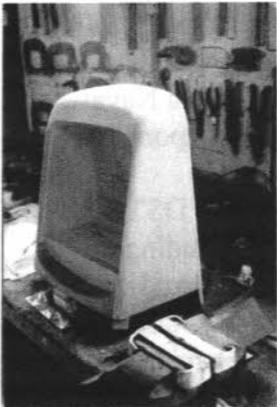
*"The radiator buck I had to make for fitting the shell."*
