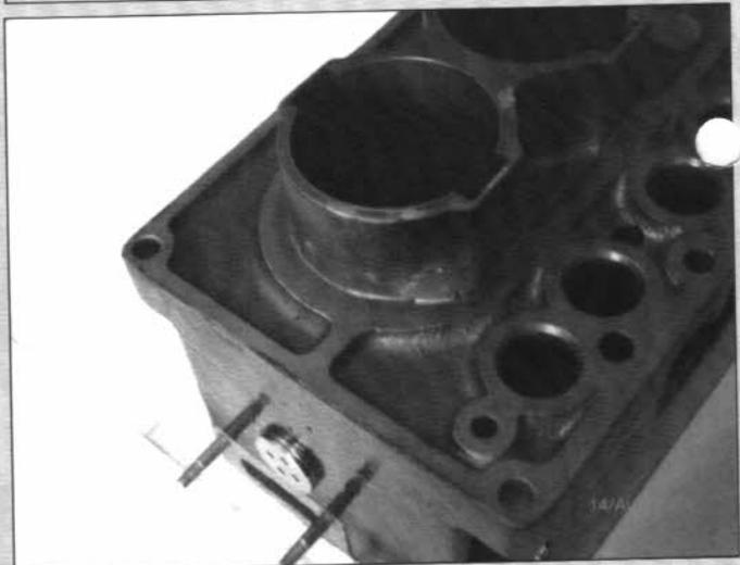
*The damaged block - brazed and dry sleeved*
