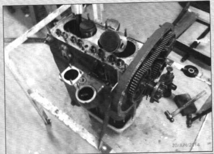
*Engine partially pulled down*
