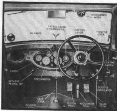
View of the Firefly's dashboard. Ample instrumentation and burled wood veneer were featured.
