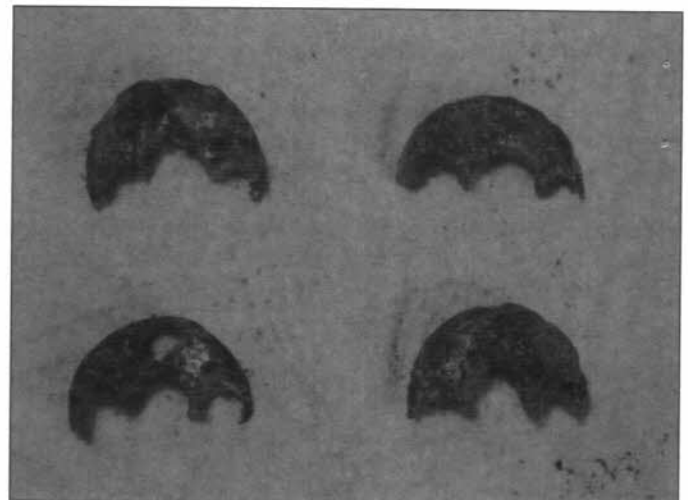
Above: Debris Below: badly corroded plugs
