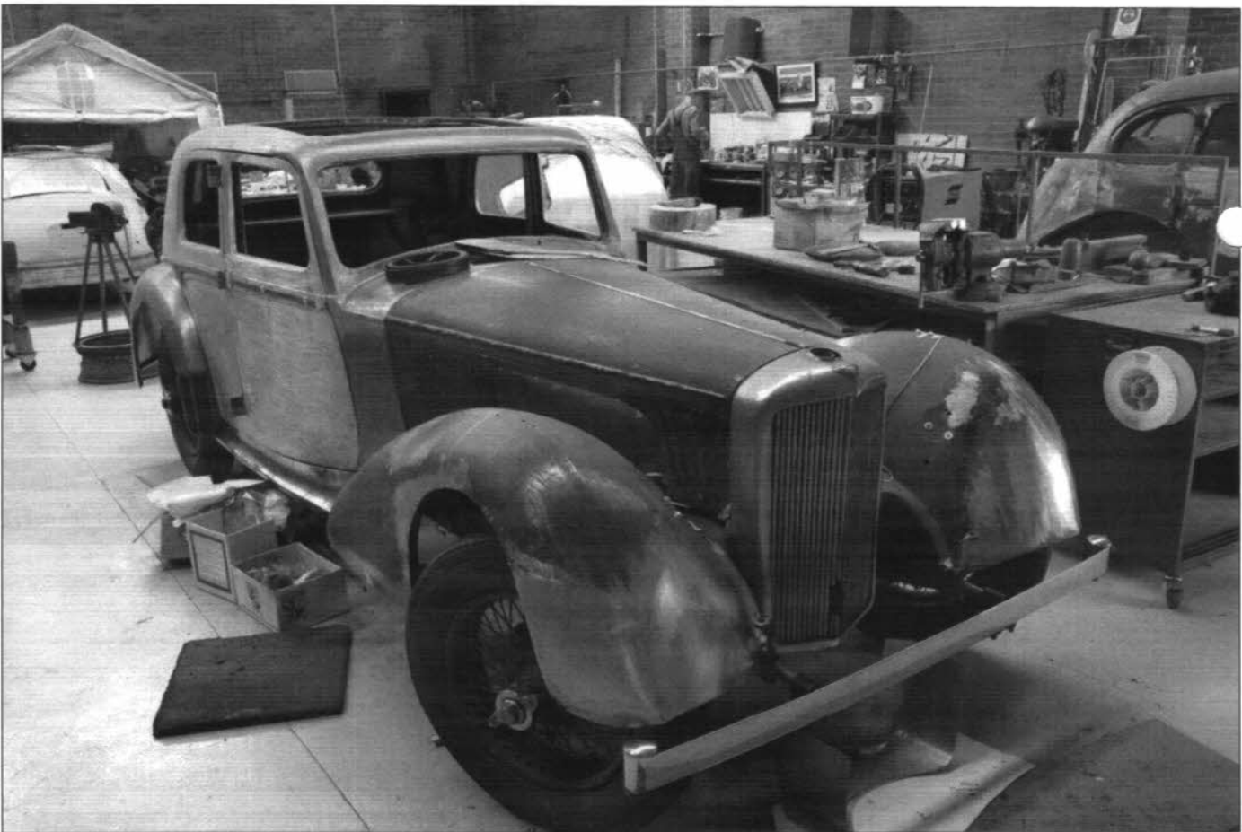
Front mudguards repaired and new front valance
