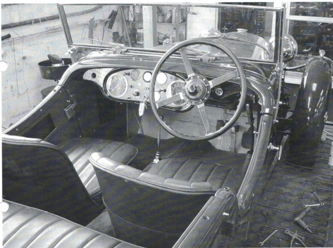
An example of the Rotax FT82 instrument panel with 5 inch speedometer and revolution counter, fitted to 1933 Model Year SA20's. Watch out for spares problems here; Follett cars were supplied with longer ignition switch control rods and instrument drives cables to accommodate his sloping instrument panels, mounted further back than those with Coventry built coachwork.
