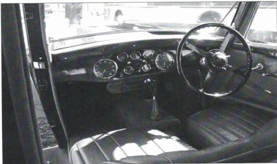
Beautifully finished instrument panel with everything in their correct places and no extra switches added. On this car, sensibly, the infamous Hobson Telegauge has been replaced with a neat dual instrument for water temperature and fuel contents.
