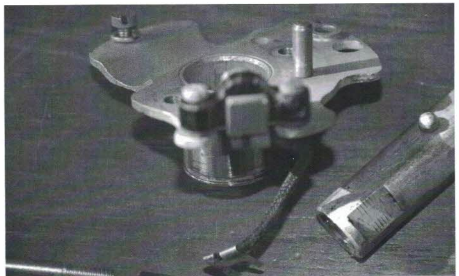
Figure 3 provides a close up of the new low tension lead and insulator "bridge". The raised hole on the right hand side of the baseplate accepts the micrometer spigot.
