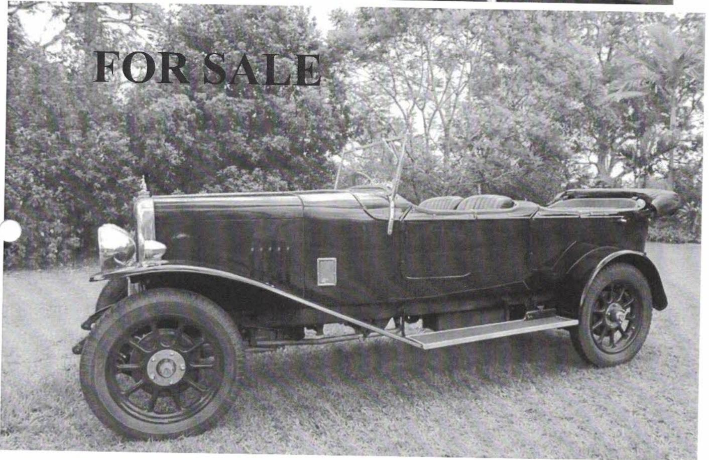
1928 14.75 Alvis Silver Eagle modified with a 16.95 engine many years ago. Chassis No 7046 Engine No 7940. Total restoration incl new replica C&E Tourer body frame. Engine total rebuild incl new pistons, rods etc. New ratio CWP 4.7:1 Sale on behalf of my daughter \$65000. Des Donnan 07 5478 6630
