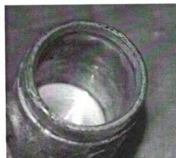
Figure 5- Near side bottom wheel cylinder. The cup was quite scored.
