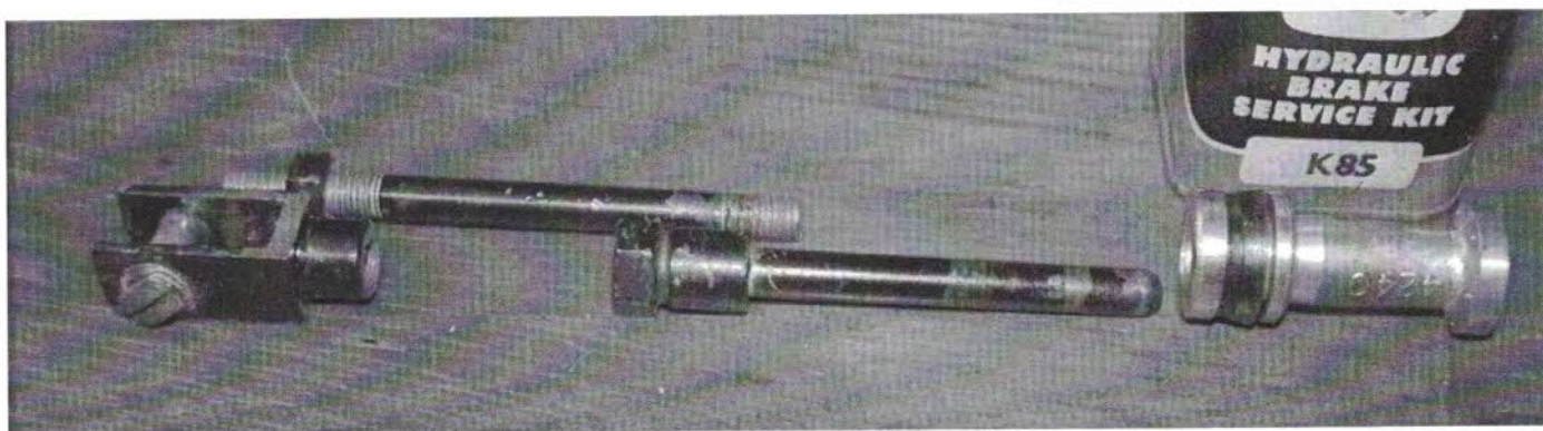
Figure 1- Linkage components and brake cylinder piston - A 1/32” play should exist between the end of the push rod and the piston when fully inserted. Prior to fitting I applied some anti-seize lubricant to the end of the push rod. See Plate I in the TA21 Catalogue of Spare Parts.
