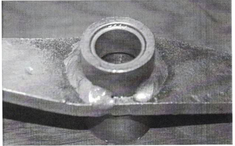
Figure 3- NOS clutch reversing lever as supplied by Red Triangle. Sintered bushes don't have the same shiny surface as do ordinary ones.
