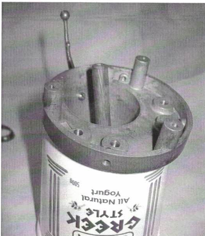
With the spindle engaged in the chassis top bearing use the dowel to help lower the assembly into the instrument body...
