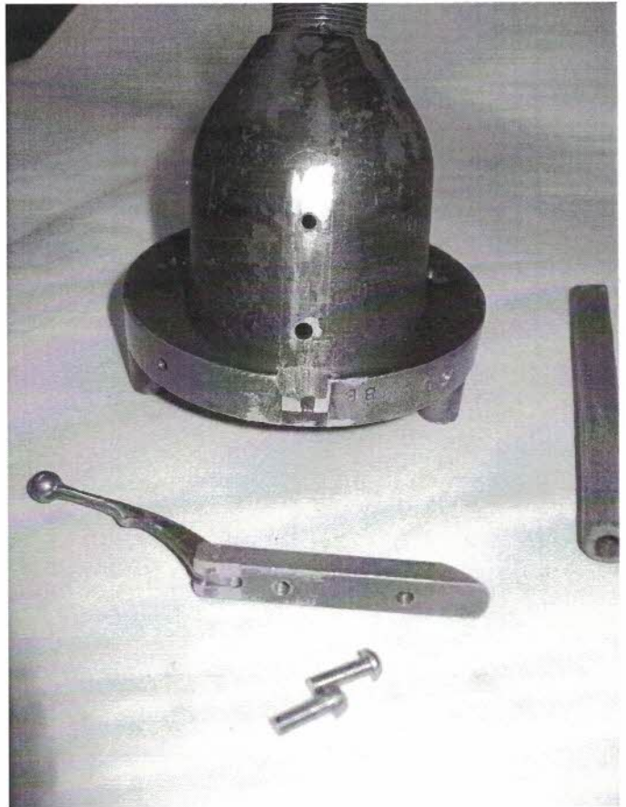
Repair of broken trip lever mount. The new steel fulcrum is fixed to the outside top of the body.
