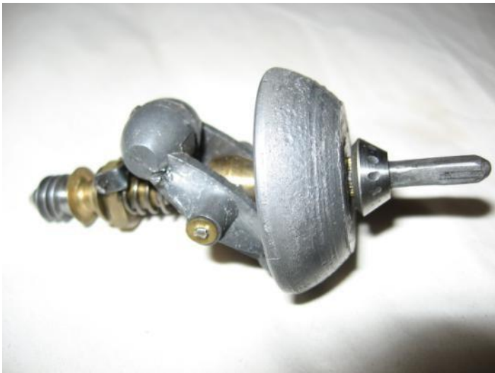
Close up of the drive spindle shows a badly pitted bearing cone (extreme right). This one is probably beyond salvage. Has any member experience of dismantling and refurbishing this pressed up assembly? The various speed ranges (60, 80, 100 etc) of the instruments are determined by the rate of the coil spring on the spindle.
